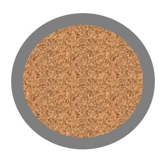
RAP aggregate with oxidized binder film
