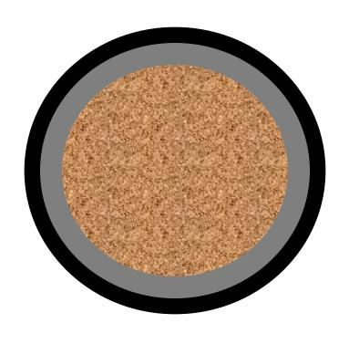
RAP aggregate with oxidized binder film plus virgin binder film
